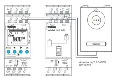
> Use 2-wire antenna cable with a maximum length of 100 m.
